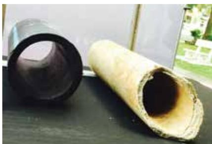
HDPE (left) and Asbestos Cement
